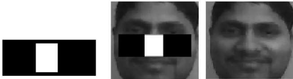
Haar-like feature applied on the bridge of the nose
